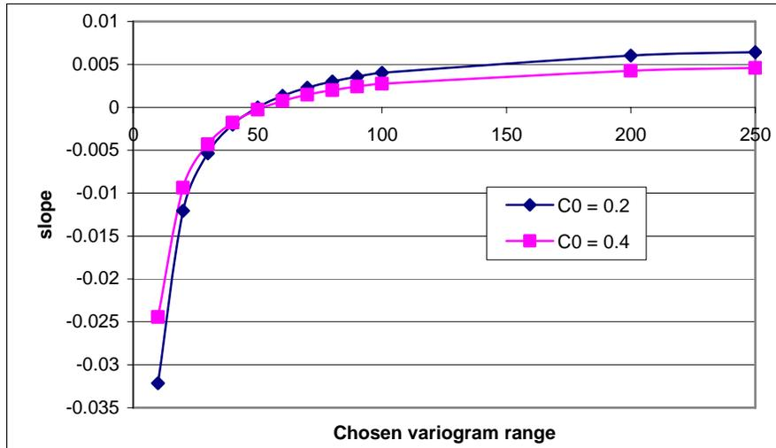
**Figure 4:** Change in the slope of the inferred nugget effect vs. composite length regression line, at different variogram ranges and for two variables simulated with nugget effect values of 0.2 and 0.4, respectively.
