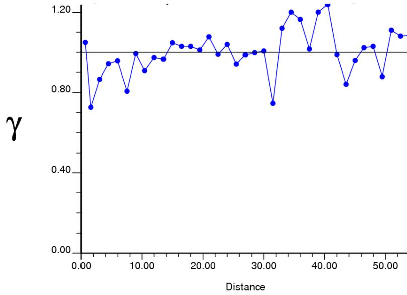
**Figure 6:** Experimental down-the-hole variogram calculated with gold assays from a disseminated deposit.
