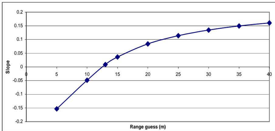
**Figure 9:** Change in the slope of the inferred nugget effect vs. composite length regression line, at different variogram ranges for gold samples.
