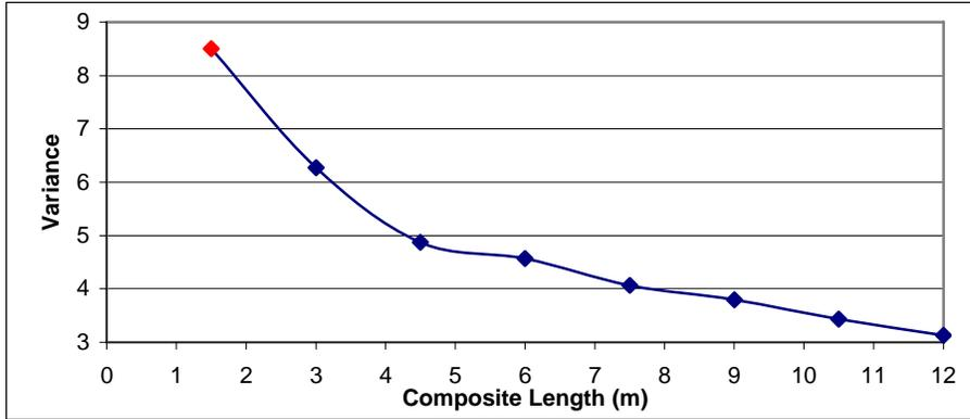
**Figure 8:** Variance of gold samples composites at different composite lengths.
