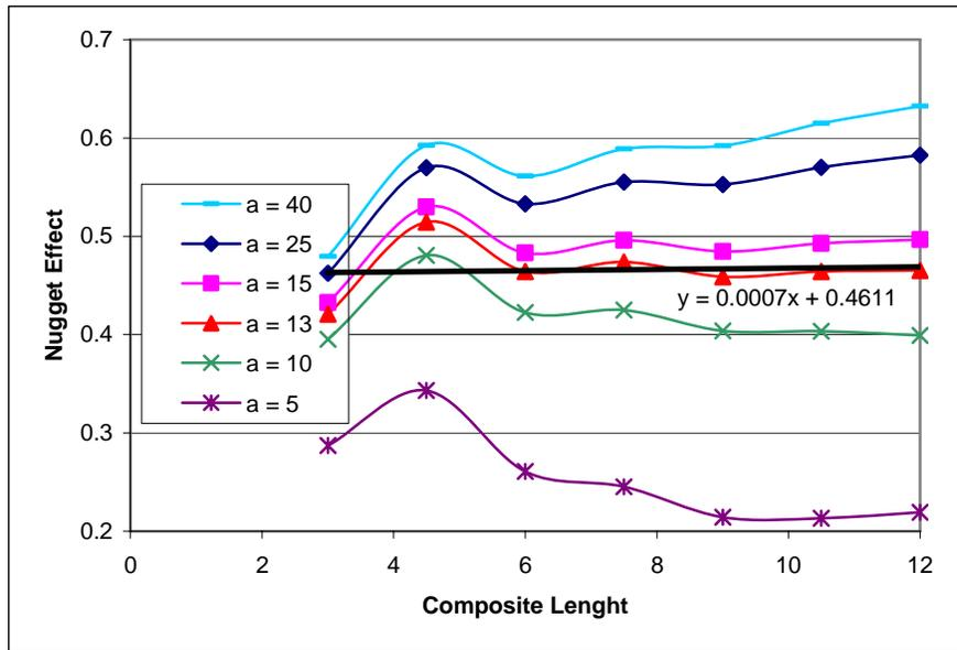
**Figure 7:** Estimated gold nugget effect values at different composite lengths and with different tentative variogram ranges.
