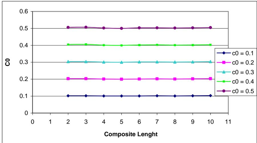
**Figure 2:** Calibrated point scale nugget effect using different composite lengths for five different variables simulated with different nugget effect values. The original sample length is 1 unit and the true variogram range is known.
