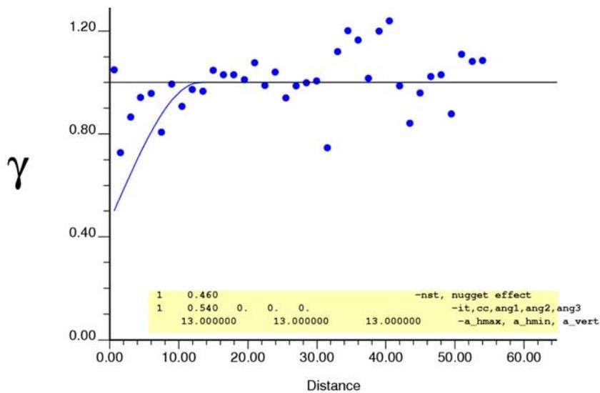
**Figure 10:** Down-the-hole gold variogram model fitted with the optimized nugget effect and variogram range parameters
